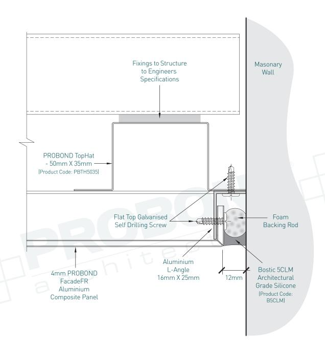
4. Detail Showing Panel at Masonary Wall
