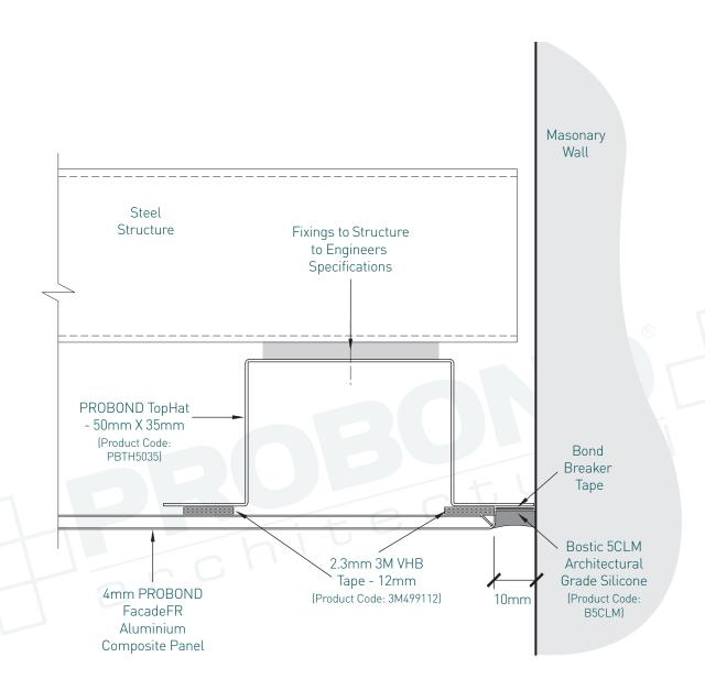
4. Detail Showing Panel at Masonary Wall
