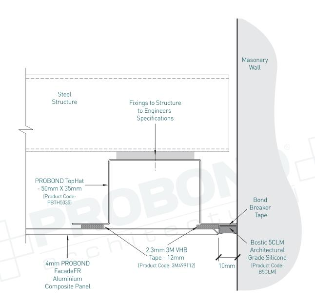
4. Detail Showing Panel at Masonary Wall
